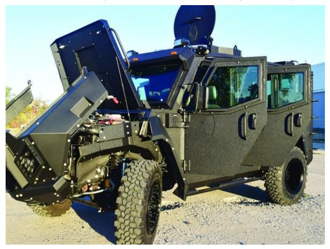
The hood design of the BATT-X facilitates maintenance. Photo: The Armored Group
